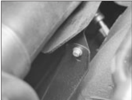
2.3 Forward air trunking to support bracket bolt
